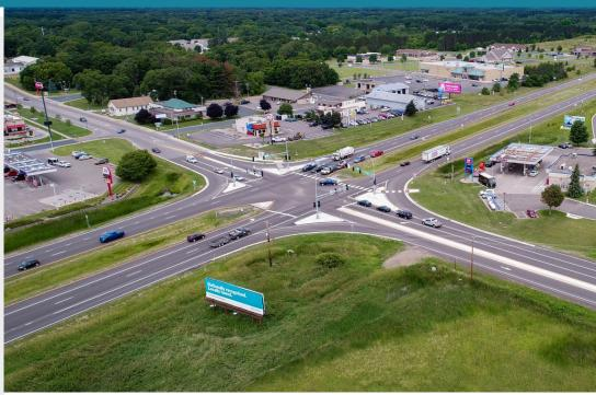
The US 169 Rural Safety and Mobility Interchange Project will reconstruct approximately one mile of US Highway 169, an existing Principal Arterial roadway, from a rural four-lane undivided highway to a four-lane divided expressway and construct a grade-separated interchange at County Road (CR) 4.
